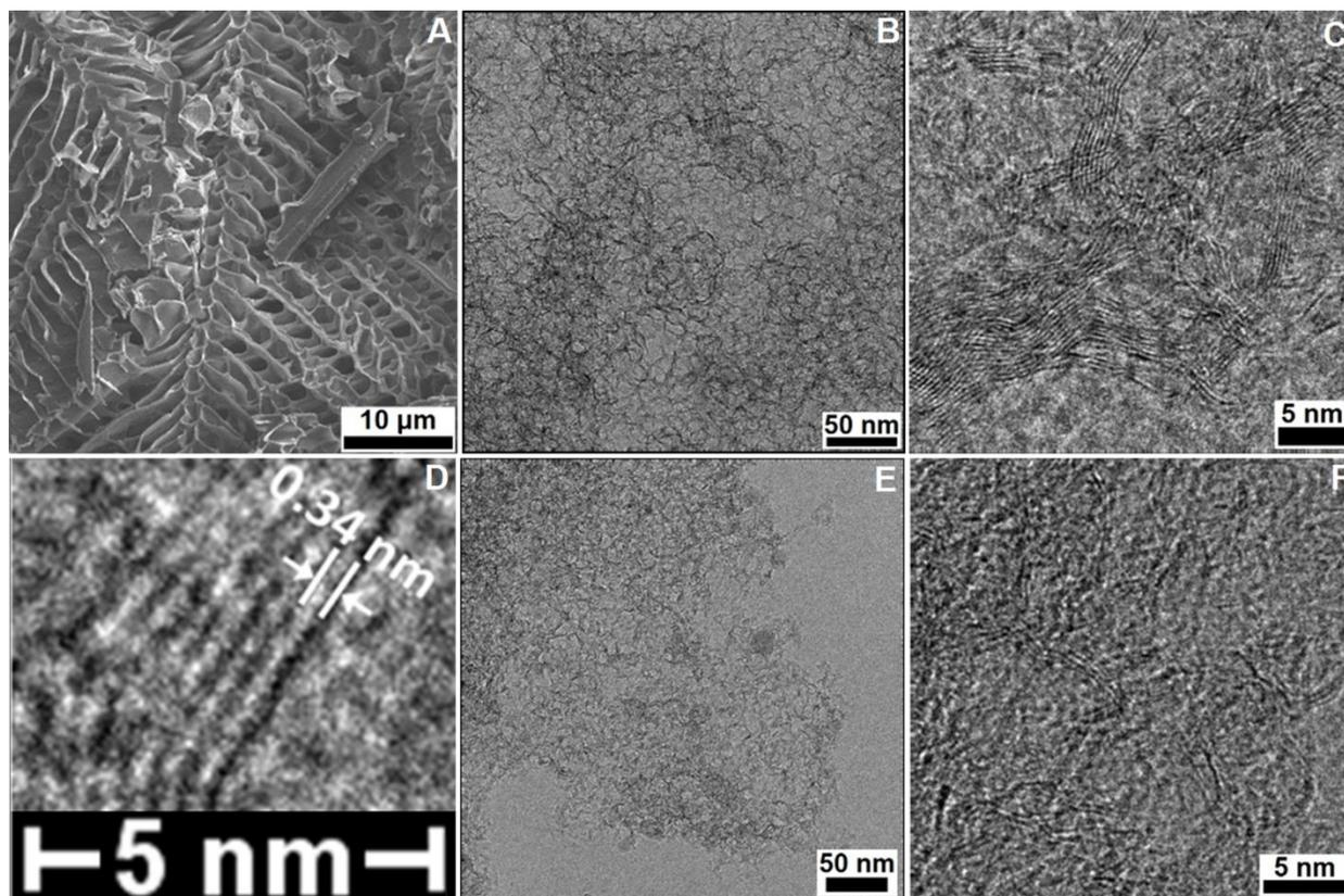
**Figure 1.** Results of electron microscopy for the HPC-G-12-21 sample reveals (a) the macroporous structure as seen by SEM and the (b) mesopores present in the macroporous walls under TEM, as well as (c,d) the graphitic ordering under HRTEM. The heavily activated HPC-G-12-21-5h sample shows (e) similar mesopores present under TEM and (f) graphitic ordering via HRTEM.
