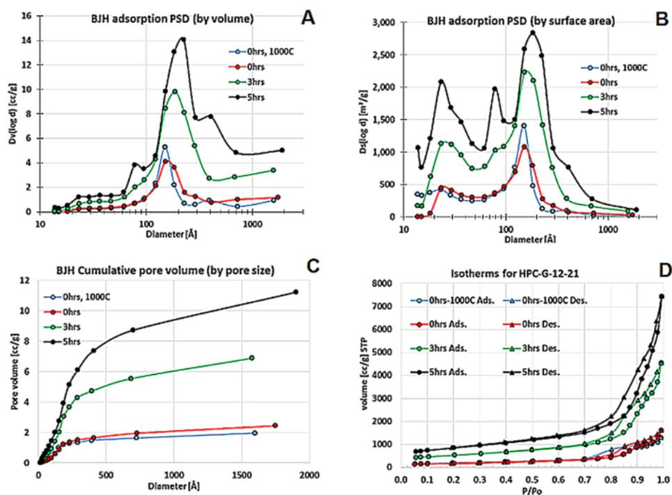
**Figure 2.** Nitrogen porosimetry data for the HPC-G materials at varying levels of activation showing (a) pore size distribution curves by volume and (b) surface area, as well as (c) cumulative pore volume as a function of pore size; all based on BJH theory. The (d) isotherms for the various levels of activation are also shown.
