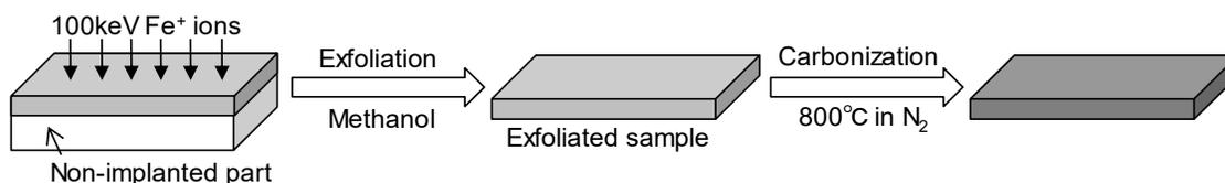
**Figure 1. Procedure of sample-preparation in this work.**
