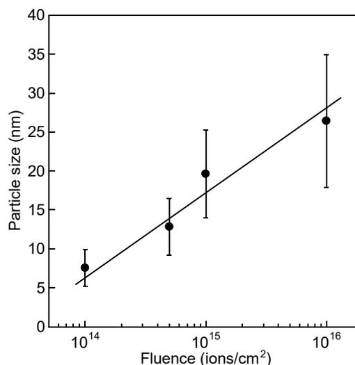
**Figure 2. Relationship between mean size of Fe nanoparticle in the obtained carbon material and fluence of 100 keV  $\text{Fe}^+$ .**
