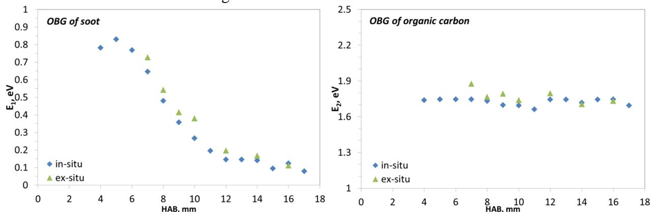
Fig.1: Optical band gap values for soot (E1, left panel) and organic carbon (E2, right panel) for ex-situ and in-situ measurements as a function of height above burner.
