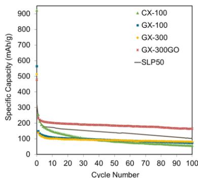
**Figure 2. Cycling performance of carbon xerogels in a Li-ion battery vs the reference material SLP50 <sup>4</sup>.**
