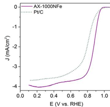
**Figure 3. LSV at 1600 rpm for a carbon xerogel in the oxygen reduction reaction vs the reference material Pt/C <sup>5</sup>.**
