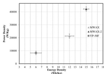
**Figure 1. Ragone plot for a supercapacitor with carbon xerogel (values calculated at  $16 \text{ A g}^{-1}$  per electrode) and aqueous electrolyte vs the reference material YP-50F <sup>3</sup>.**
