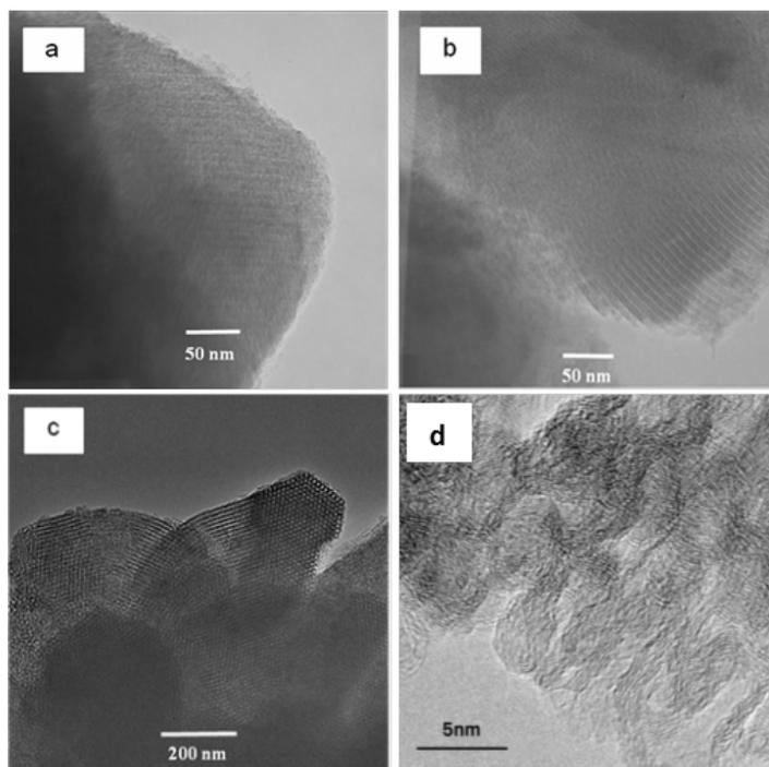
Figure 1. TEM images of SBA-15 (a), active SBA-15 (b) and NMTC (c) and (d)
