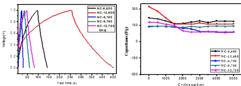
Figure 3. Charge/discharge curves and cycling lives
