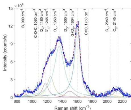
Fig. 1: Raman spectral deconvolutions of non-heat treated OP6 soot
