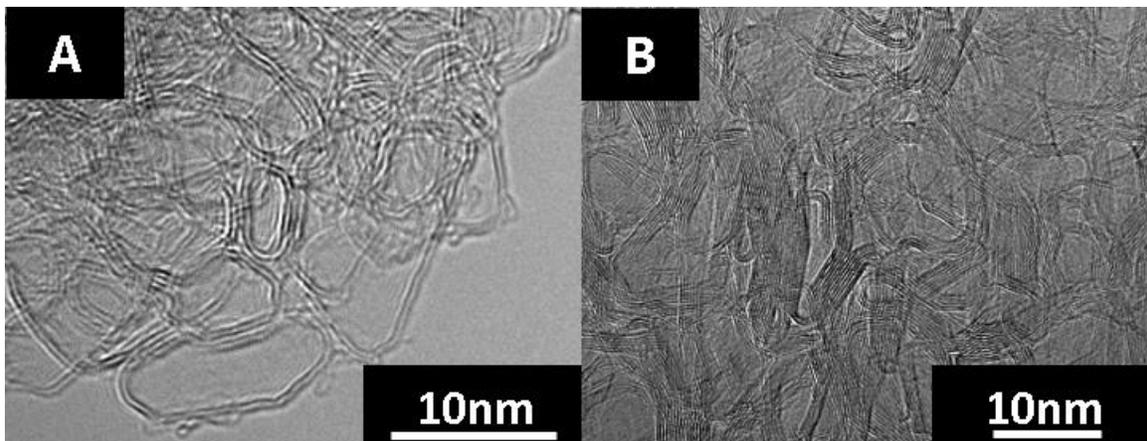
**Figure 1.** TEM micrograph of CO<sub>2</sub> laser annealed sucrose char. A) after 5 seconds, B) After 20 seconds.
