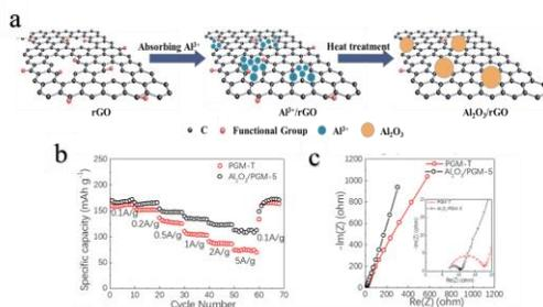
**Figure 2.** a) Scheme of the formation of  $\text{Al}_2\text{O}_3$  nanoclusters on defective rGO, b) Rate performance and c) EIS comparison of electrodes with or without  $\text{Al}_2\text{O}_3$  nanoclusters shielding.
