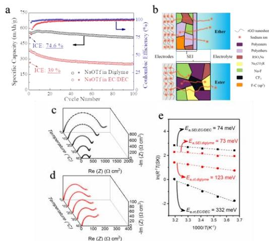
**Figure 1.** a) the comparison of electrochemical performance, b) the scheme for the different composition of SEI and c) temperature-dependent EIS of rGO electrodes in different electrolytes.
