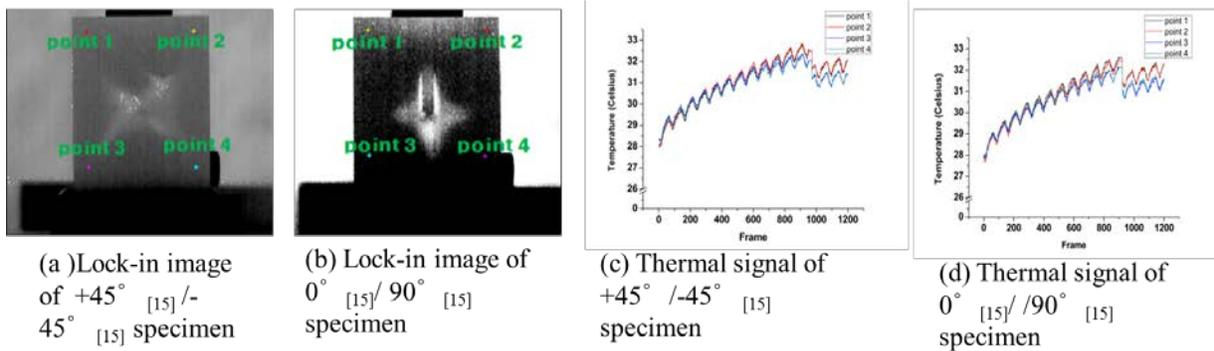
**Figure 3 Results of Lock-in non-destructive Testing**
