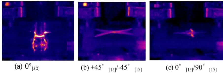
**Figure 2 Drop-weight Test of each specimen**
