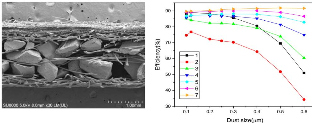
**Figure 2. Cross section SEM image and filter efficiency results of the filter media**
