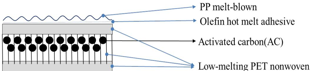
Figure 1. The structure of AC filter media
