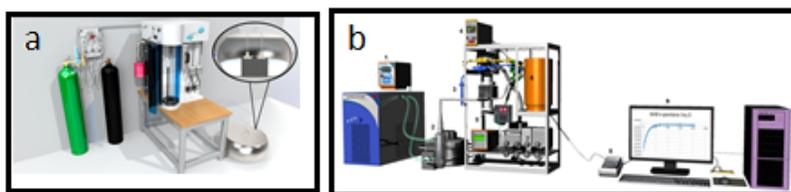
**Figure 1.** a) Adsorption calorimetry set-up used to determine the differential heat of adsorption of alcohols on MOFs
