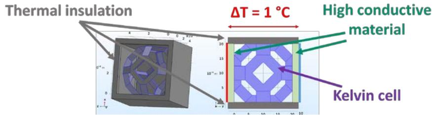
Figure 2. 3D geometry of the model, and boundary conditions.
