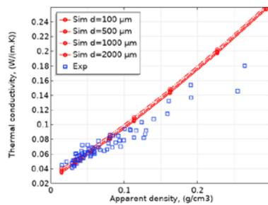
Figure 3: Evolution of thermal conductivity with apparent density
