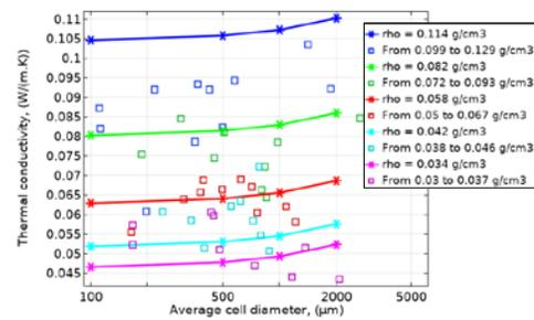
Figure 4: Evolution of thermal conductivity with average cell diameter
