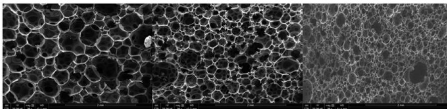
**Figure 1.** SEM images (secondary electron detector) of Standard carbon foams (magnification  $\times 30$ ) of apparent densities (from left to right) 0.043, 0.051 and 0.111 g cm<sup>-3</sup>.
