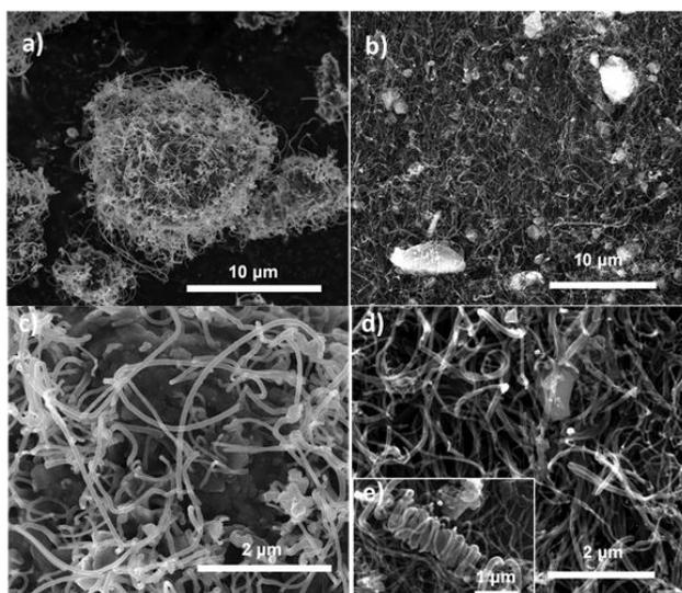
**Figure 2.** SEM images of the samples synthesized from samples 1H (a, c) and 1H-Ox (b, d) at 5,000X and 25,000X.
