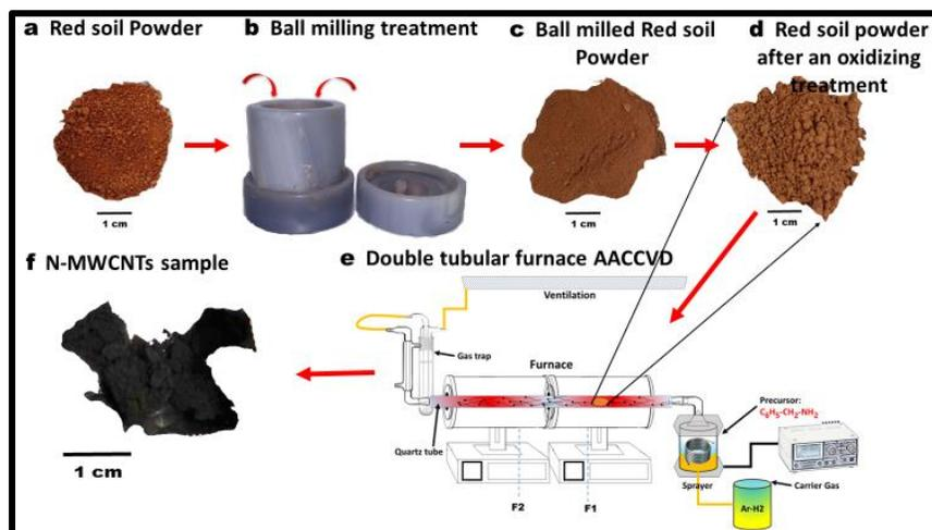
**Figure 1.** Schematic representation of the steps followed for the production of N-MWCNTs using a Leptosol enriched in Fe as catalysts. (a) Pristine soil, (b) Mechanical grinding treatment, (c) Soil after milling, (d) soil after oxidation treatment, (e) AACVD system, (f) N-MWCNT.
