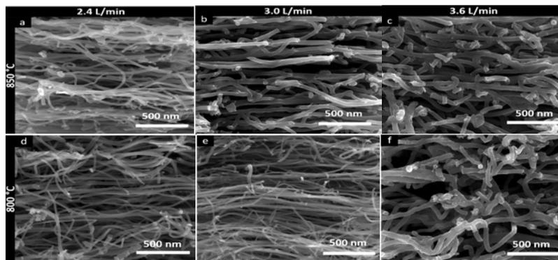
**Figure 1. Images of SEM for N-MWCNTs grown at 800 °C and 850 °C for three different entrainment flows.**
