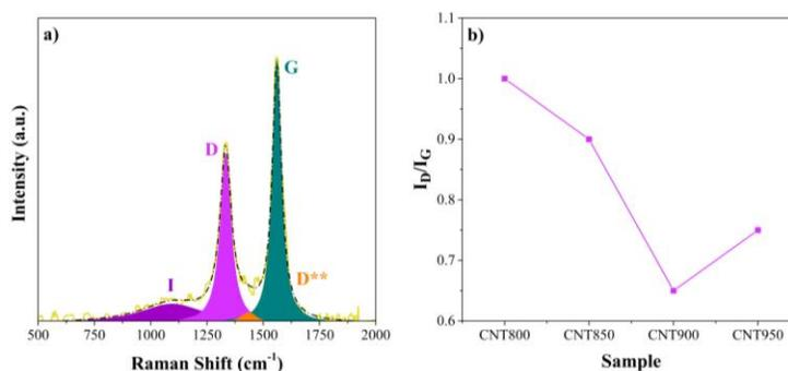
**Figure 2.** a) Deconvolution of Raman bands for sample CNT900 showing bands I, D, G and D\*\* that can be associated with the incorporation of N,  $sp^2$  network defects, C-C stretching and staking imperfections, respectively, b)  $I_D/I_G$  ratio vs sample.
