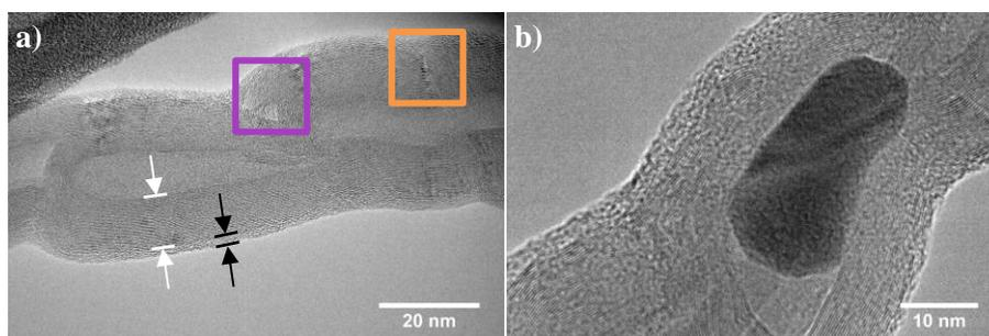
**Figure 1.** TEM image from sample CNT900, a) a N-MWCNT showing wavy walls, staking defects (violet square), strains (orange square), graphitic-like core (white arrows) and amorphous-like external walls (black arrows), b) a Ni particle inside a N-MWCNT.
