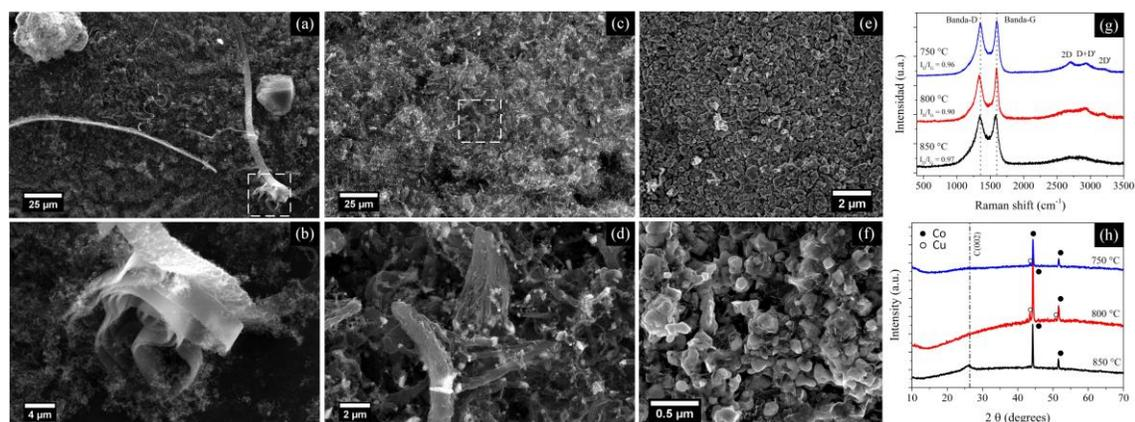
**Figure 1:** a-b) CNT grown over Wrinkled Carbon Belts at 850 °C. c-d) Defected wrinkled belt structure obtained at 800 °C. e-f) Cu-Co NPs surrounded by graphitic material obtained at 750 °C. g) Raman spectra of samples obtained at 750 °C, 800 °C and 850 °C. h) XRD diffraction pattern of samples obtained at 750 °C, 800 °C and 850 °C.
