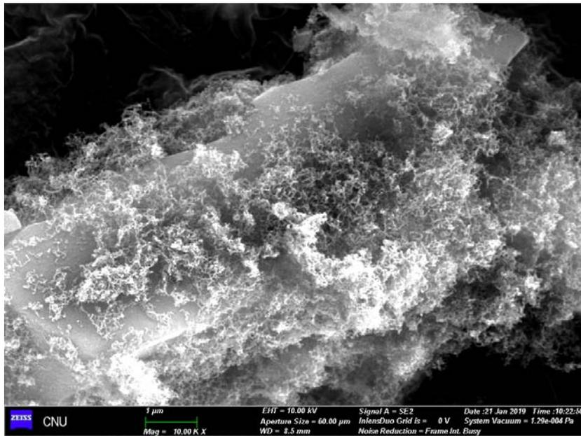
**Figure 1. SEM image of metal - impregnated porous nano carbon composites**
