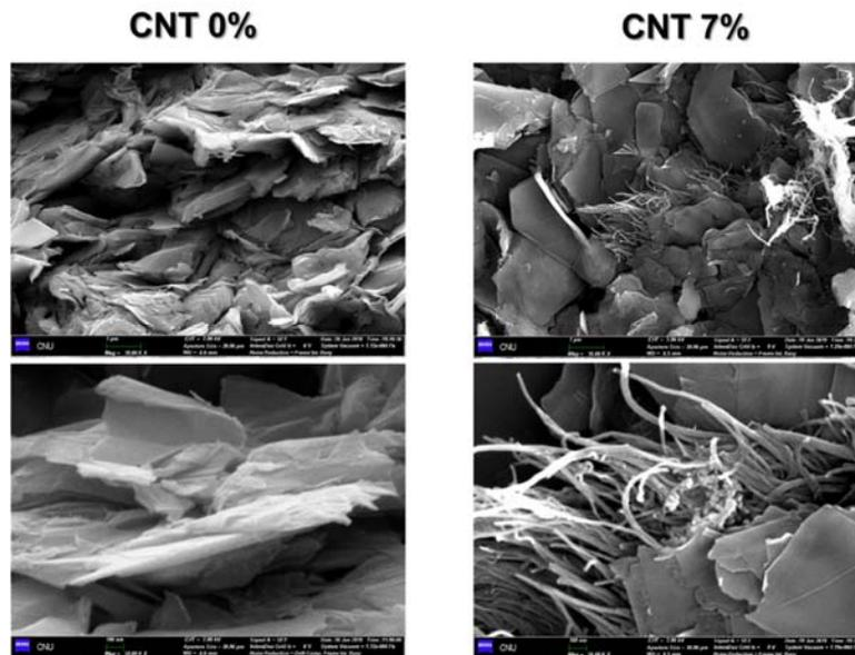
Figure 1. SEM image of CNT /graphite/epoxy nano composite bipolar plates
