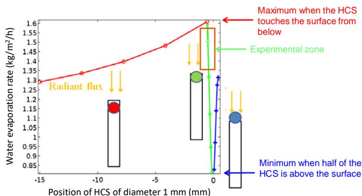
**Figure 1. Simulated change of evaporation rate produced by one HCS submitted to 1 kW/m<sup>2</sup> of solar energy, as a function of its position in the water column.**
