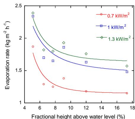
**Figure 2. Measured evaporation rate under three different solar energy densities, as a function of floatability.**
