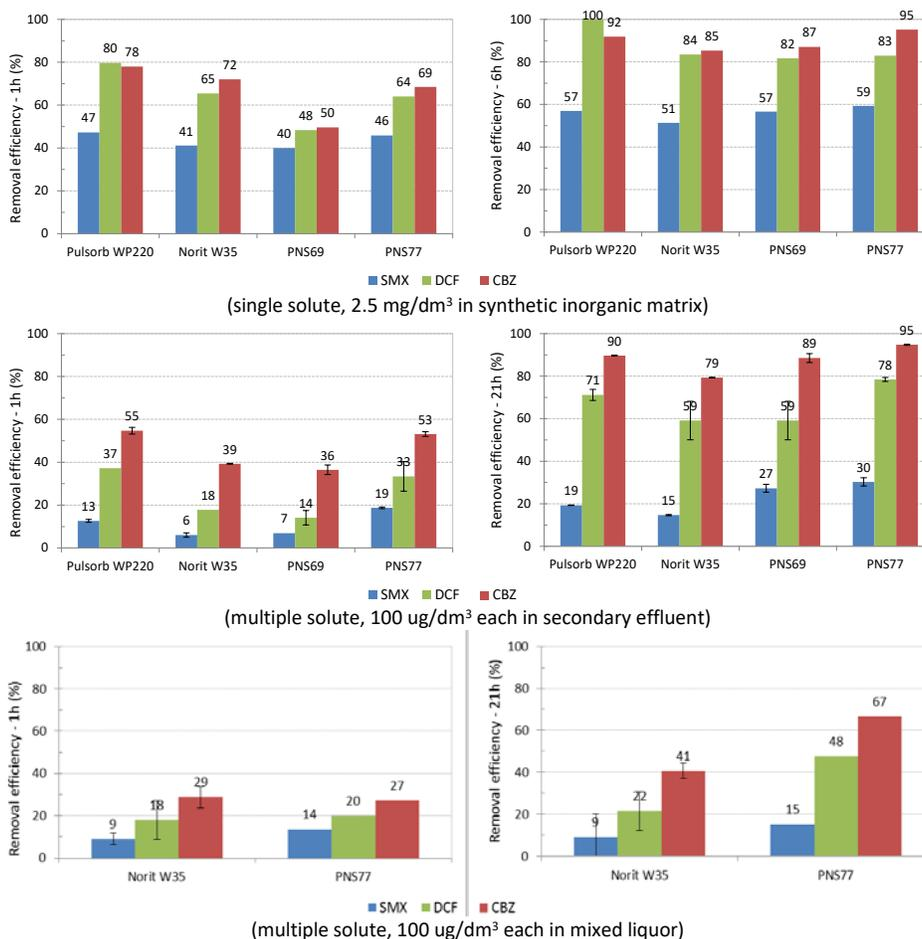
**Figure 1. Removal efficiencies of the four tested PACs for the target PhCs (top) in synthetic inorganic matrix spiked with 2.5 mg/dm<sup>3</sup> of each PhC in single-solute conditions and (middle) in secondary effluent spiked with 100 µg/dm<sup>3</sup> of each PhC in multi-solute conditions and of Norit W35 and PNS77 (bottom) in mixed liquor spiked with 100 µg/dm<sup>3</sup> of each PhC in multi-solute conditions**
