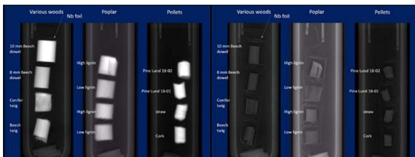
Fig. 1 InA images of different wood and pellet samples wrapped in Nb foil inside alumina tubes before (left frame) and after (right frame) pyrolysis at up to 1000 °C.
