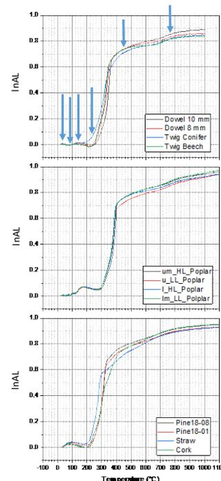
Fig. 3 Work-In-Progress on data evaluation of InAL and H loss with temperature. Real maximum temperature was 1000 °C. 0: start; 1–5: regions of special interest.
