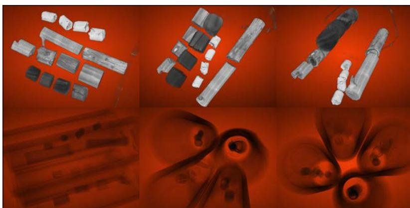
Fig. 2 NCTs on all sample tubes. Fresh samples (top row), pyrolyzed samples (bottom row).
