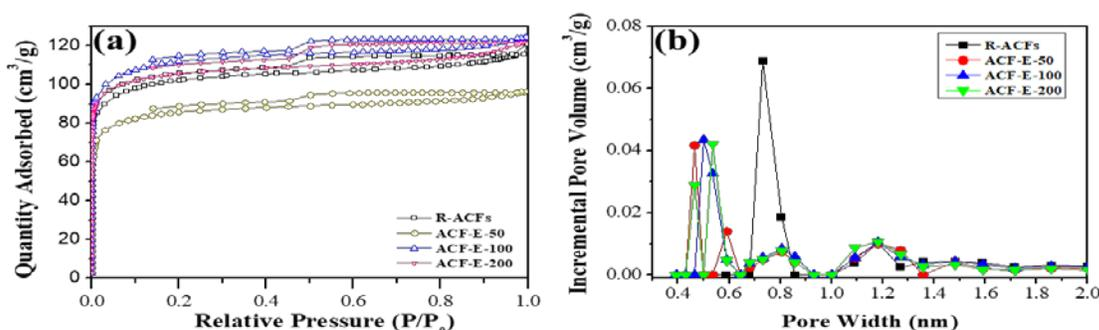
**Figure 1. Nitrogen adsorption-desorption and pore size distribution plots of untreated and E-beam-treated ACFs.**
