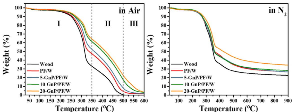
**Figure 1. TGA curves of GnP/re-PF/W composite boards analyzed under air and N<sub>2</sub> atmosphere.**
