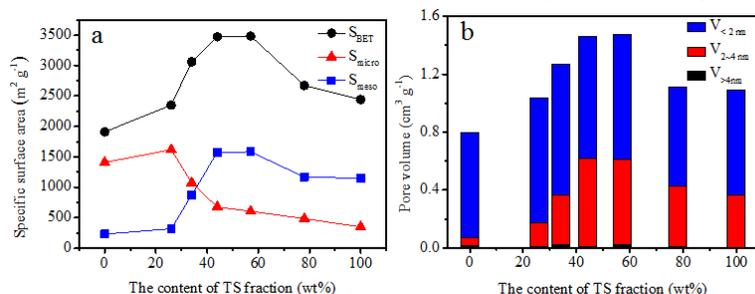
**Figure 1. The relationship between the content of TS fraction in the precursor and the specific surface area (a) and pore volume (b) of PACs.**
