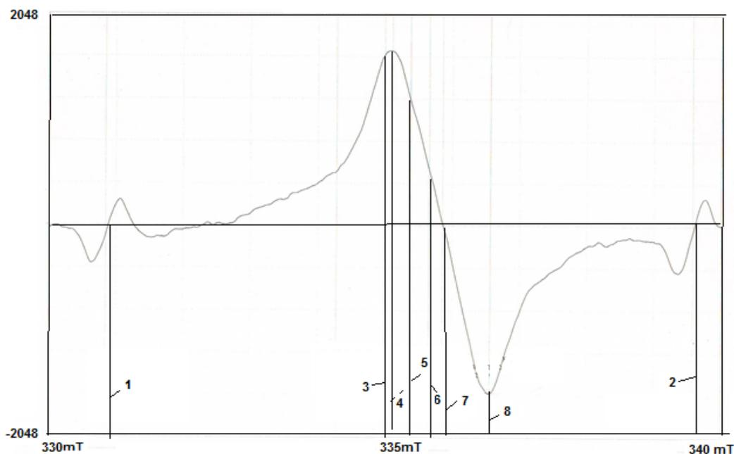
Fig.1 The EPR spectrum of graphen structures obtaining by under the influence of an ultrasonic field on graphite with aromatic hydrocarbons (toluene) at treatment of 30 minute
