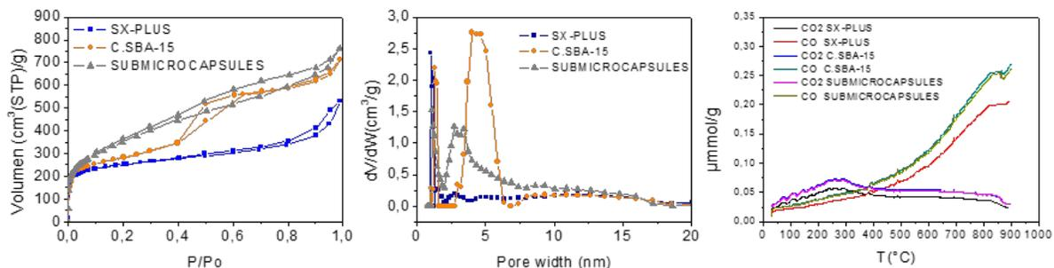
**Figure 1.** a) N<sub>2</sub> adsorption-desorption isotherm at 77 K and b) pore width distribution and c) Temperature programmed desorption of carbon samples
