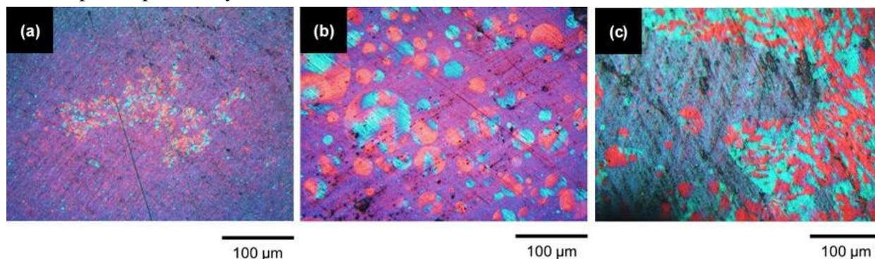
**Figure 1.** Anisotropic structure of the obtained pitches after N<sub>2</sub> blowing heat-treatment; (a) EBOp-Br, (b) (EBOp/CTP)-Br and (c) (EBOp/FCC-DO)-Br.
