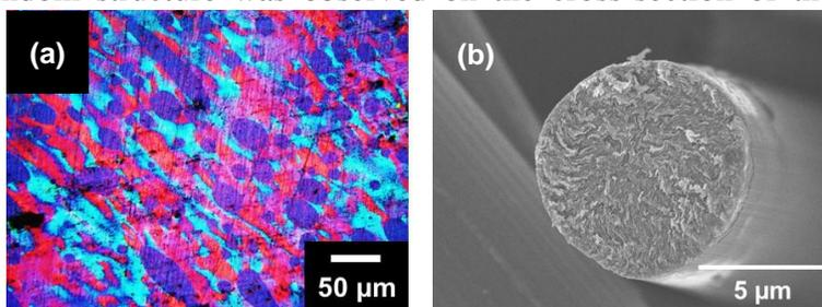
**Figure 1. (a) Anisotropic structure of HPC-derived mesophase pitch and (b) SEM image of HPC-derived MPCF after graphitization.**
