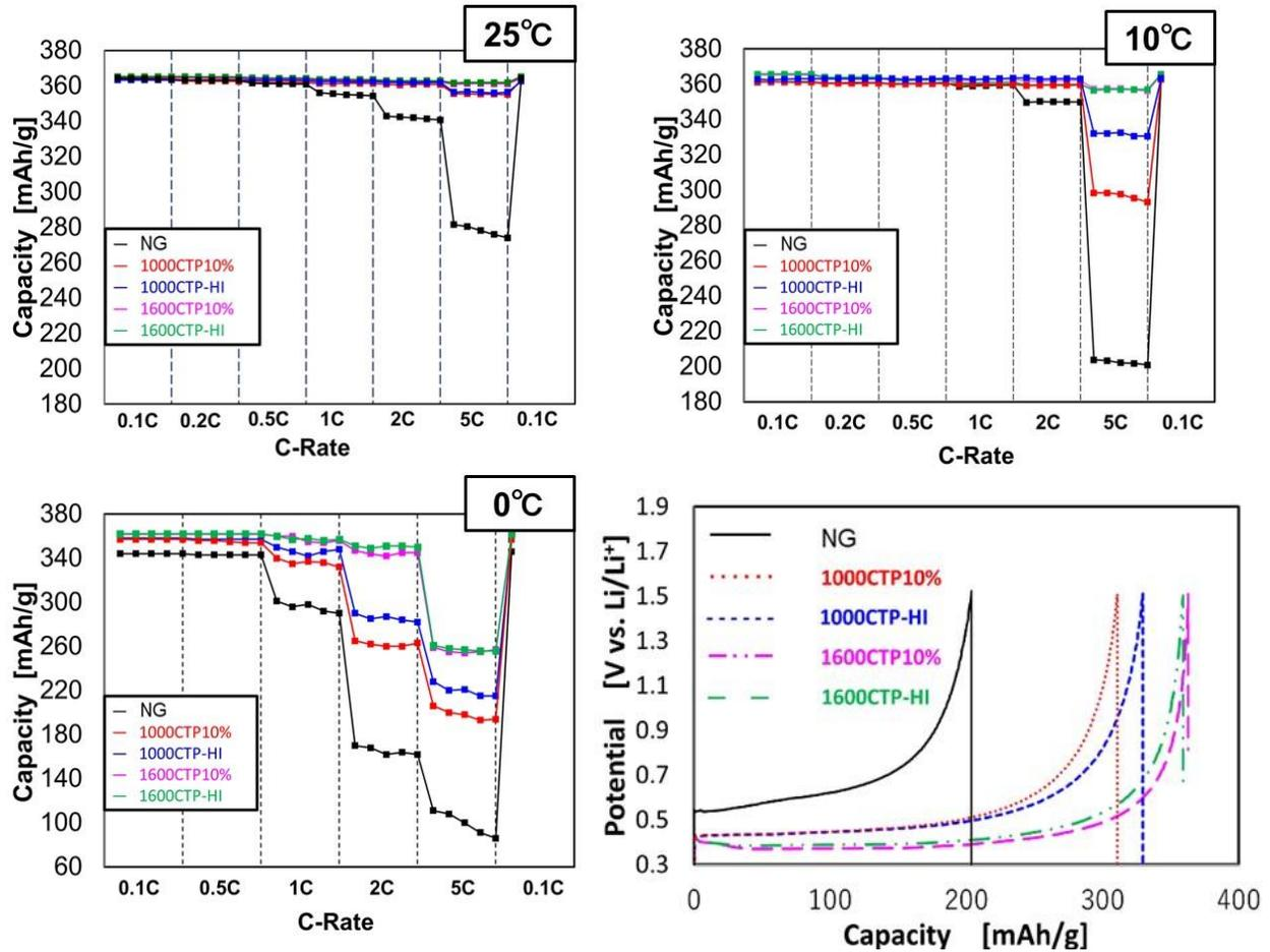
Figure 1. Rate performance at various temperature and discharge curves at 10°C using NG coated amorphous carbon.
