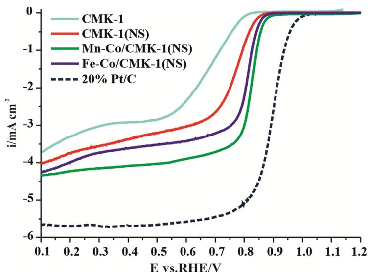
**Figure 1.** LSV curves of spinel catalysts deposited on N, S-doped mesoporous carbon support in  $\text{O}_2$ -saturated  $0.1 \text{ M KOH}$  solution recorded at 1600 rpm.
