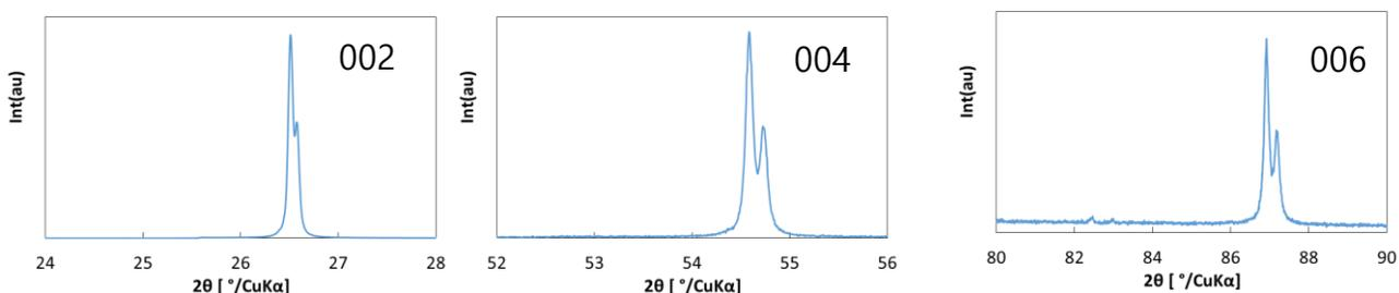
**Figure 2** X-ray diffraction lines with 00L indices from the reflection configuration to the graphitized film surface.
