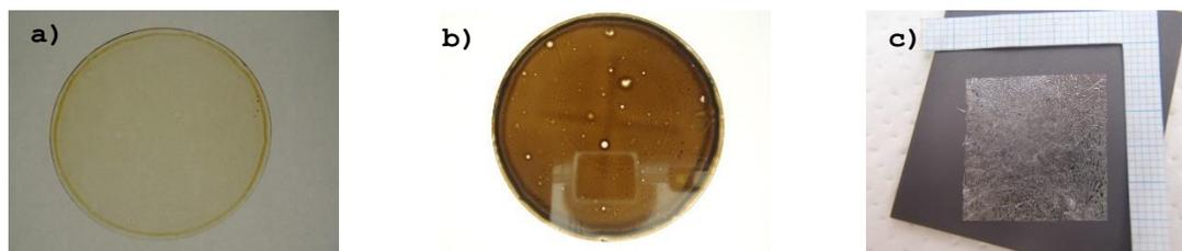
**Figure 1** Photographs of the film produced from sucrose solution: a) caramelized with substrate at 180 °C in air, b) carbonized with substrate at 600 °C in nitrogen and c) graphitized in between graphite plates under argon atmosphere at 2800 °C.
