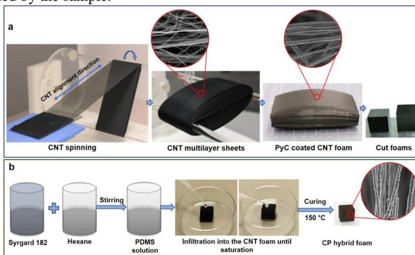
**Figure 1.** Schematic of (a) CNT/C (C-100) foam fabrication and (b) CNT/C-PDMS (CP) hybrid foam preparation process
