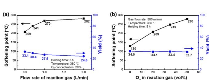
**Figure 2.** Softening point and yield variation of pitches prepared by oxidative thermal treatment as a function of (a) flow rate of the reaction gas and (b) O<sub>2</sub> concentration in the reaction gas.
