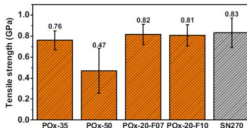
**Figure 1.** Tensile strength of carbon fibers prepared from the experimental pitch samples (POx-35, POx-50, POx-20-F07 and POx-20-F10) and commercial isotropic pitch (SN-270).
