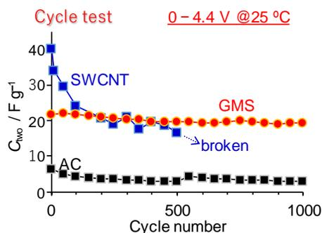
**Figure 4.** The capacitance change of each sample during cycle test at 4.4 V and 25 °C.
