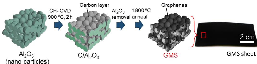
**Figure 1.** The preparation scheme of GMS and a photograph of a GMS sheet.
