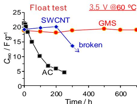
**Figure 3.** The capacitance change of each sample at 3.5 V and 60 °C.
