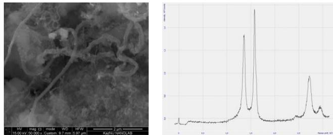
**Figure 2 - SEM image and Raman spectra of carbon nanotubes at different scales synthesized on Ni/NiO@sp-Al<sub>2</sub>O<sub>3</sub>**
