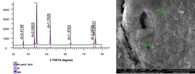
**Figure 1 – XRD-pattern and SEM image of a Ni/NiO sample**
