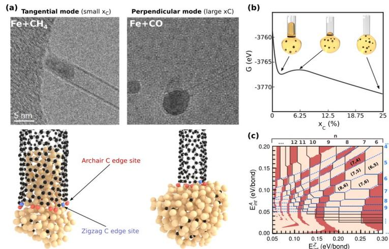
**Figure 1.** a) TEM images and simulated tangential and perpendicular growth modes depending on carbon concentration inside the catalyst. b) Free energy depending on carbon concentration. Chirality diagram depending on contact energy between zigzag and armchair C edge sites with a Ni catalyst. Brown area denotes metallic (n,m) tubes chirality, light grey denotes semiconducting (n,m) tubes chirality.
